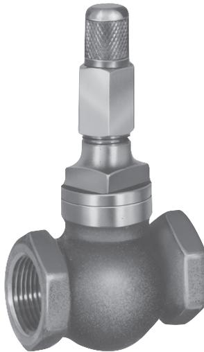
Eclipse Adjustable Limiting Orifice Valves are recommended for installation in gas lines feeding nozzle mix burners as a means of gas flow adjustment for the desired air / gas ratio. The unique V-port design allows for extremely fine ratio adjustment.
